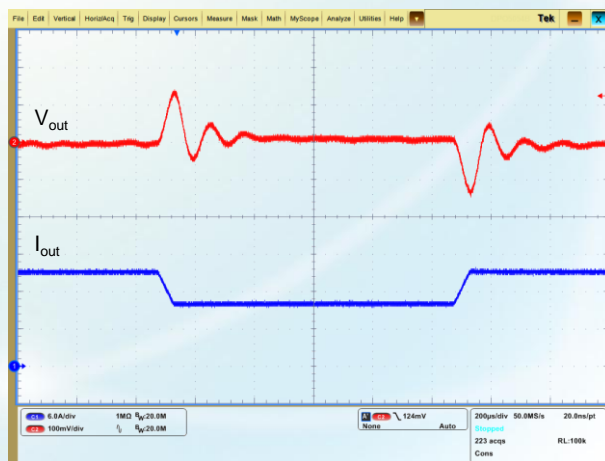
Figure 16: Output voltage dynamic response (Load: 50% - 75% - 50%, di/dt = 0.1\text{ A}/\mu\text{s} )
